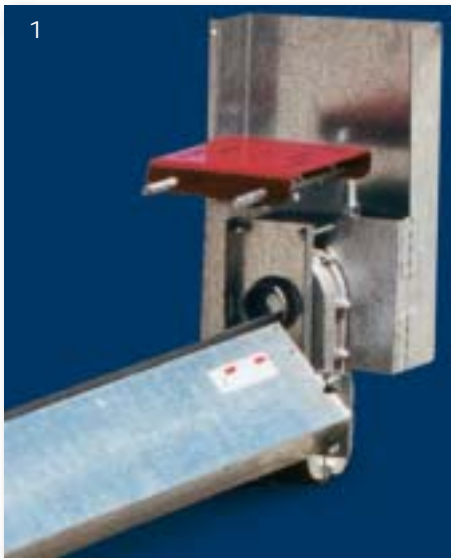
Photo 1: The Klean Sweep drive consists of a heavy duty motor mount and a cast aluminum housing, enclosing the chain and sprockets in oil.
