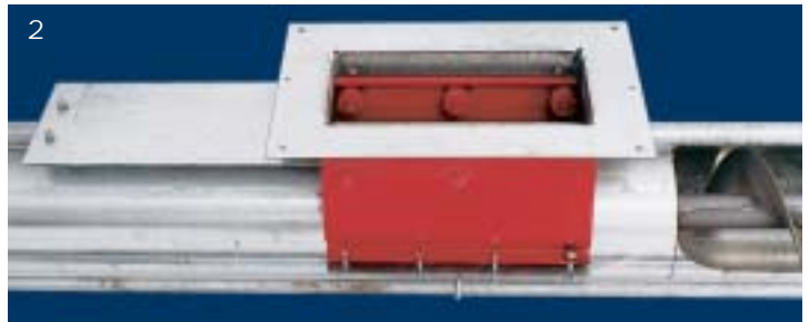
Photo 2: Both center and intermediate wells feature exterior gate control. The control pipe and lever system includes pipes that control the clutch and all wells plus outside levers and hardware.
