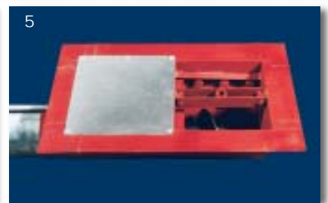
Photo 4 & 5: Bin wells have 1/4" plate steel gates supported by rollers; Gates slide into chambers protected from grain weight. May be used under suspended floor, in a trench or cast in concrete.
