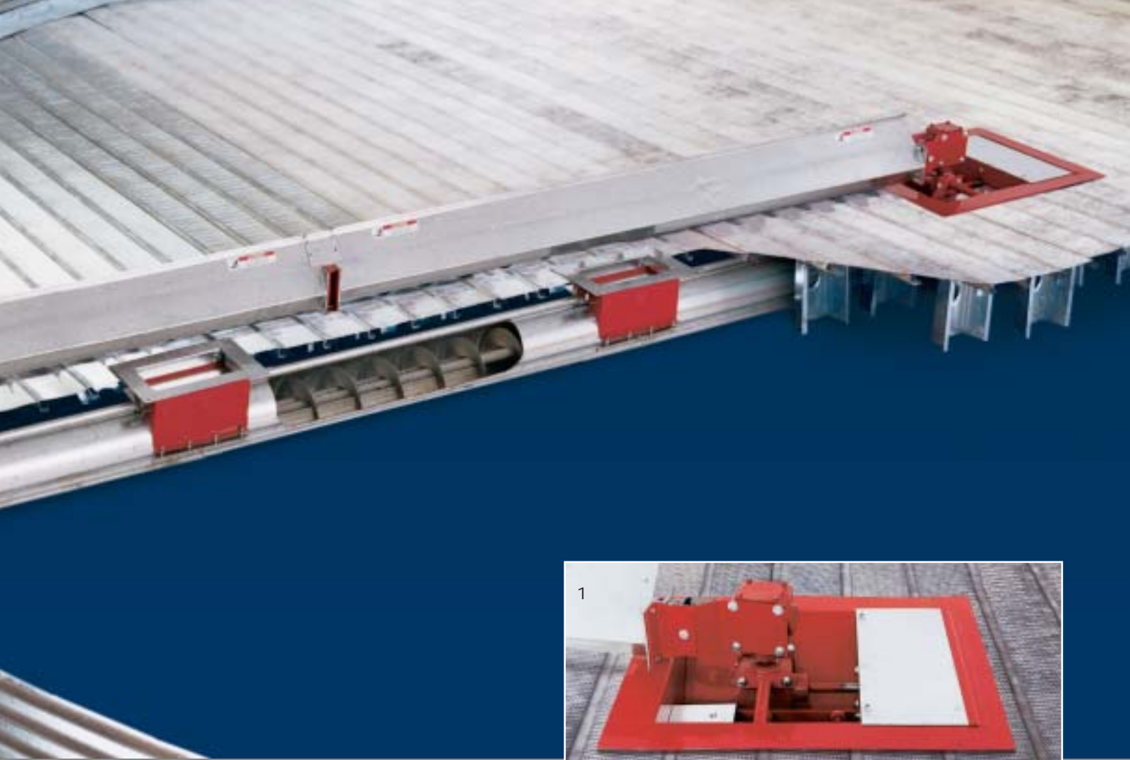
Photo 1: The center well is equipped with a double gear box assembly to transmit power from the under-bin auger to the sweep.
